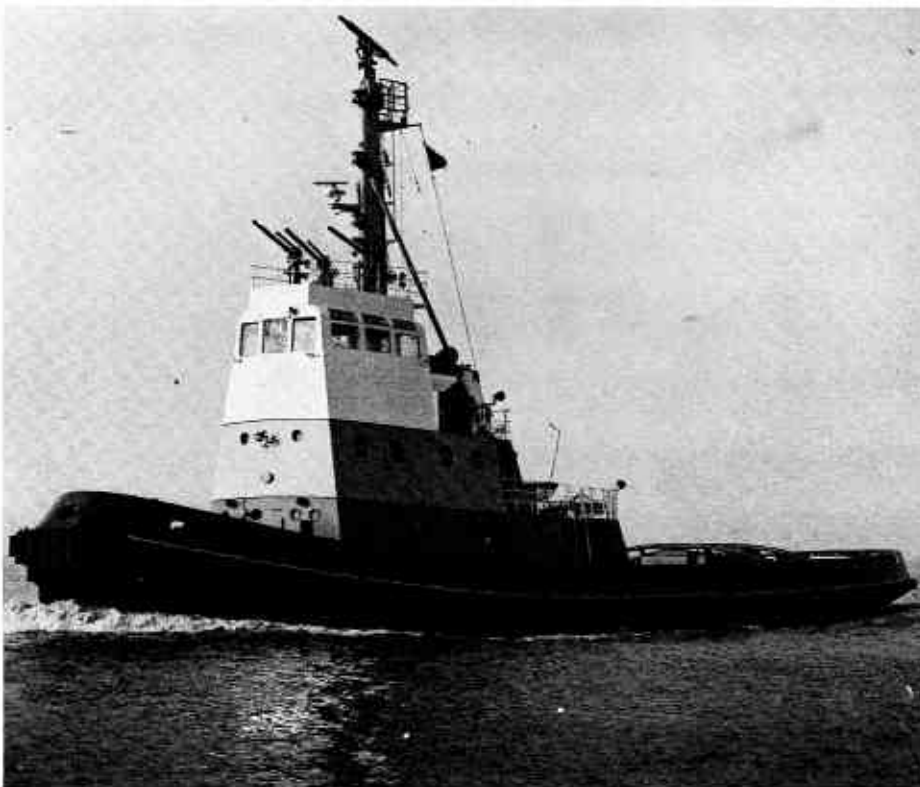
Typical of the tugs which handle supertankers. This is 'Point Gilbert' a fire fighting tug which has a 12 RKCM engine at 900 revs/min.
